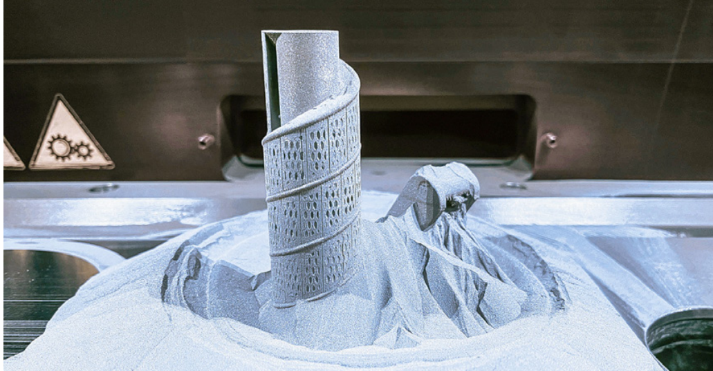
Complex functional metal part produced with powder bed fusion (PBF-LB/M) comprising inner structures which could not be produced with conventional manufacturing.
