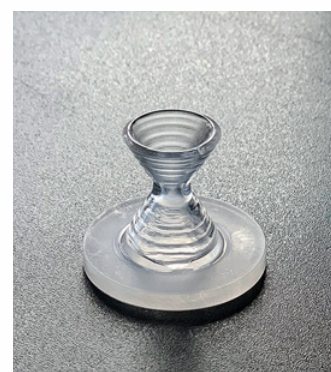
Sandglass structure printed with the LGD process.
