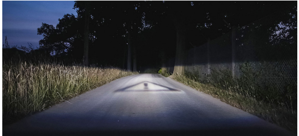
High-resolution vehicle headlamps can project symbols onto the street surface to communicate with the driver or other road users.
