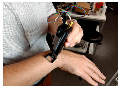
A measuring probe of the optical system to detect skin cancer. It is being further developed for clinical use.
