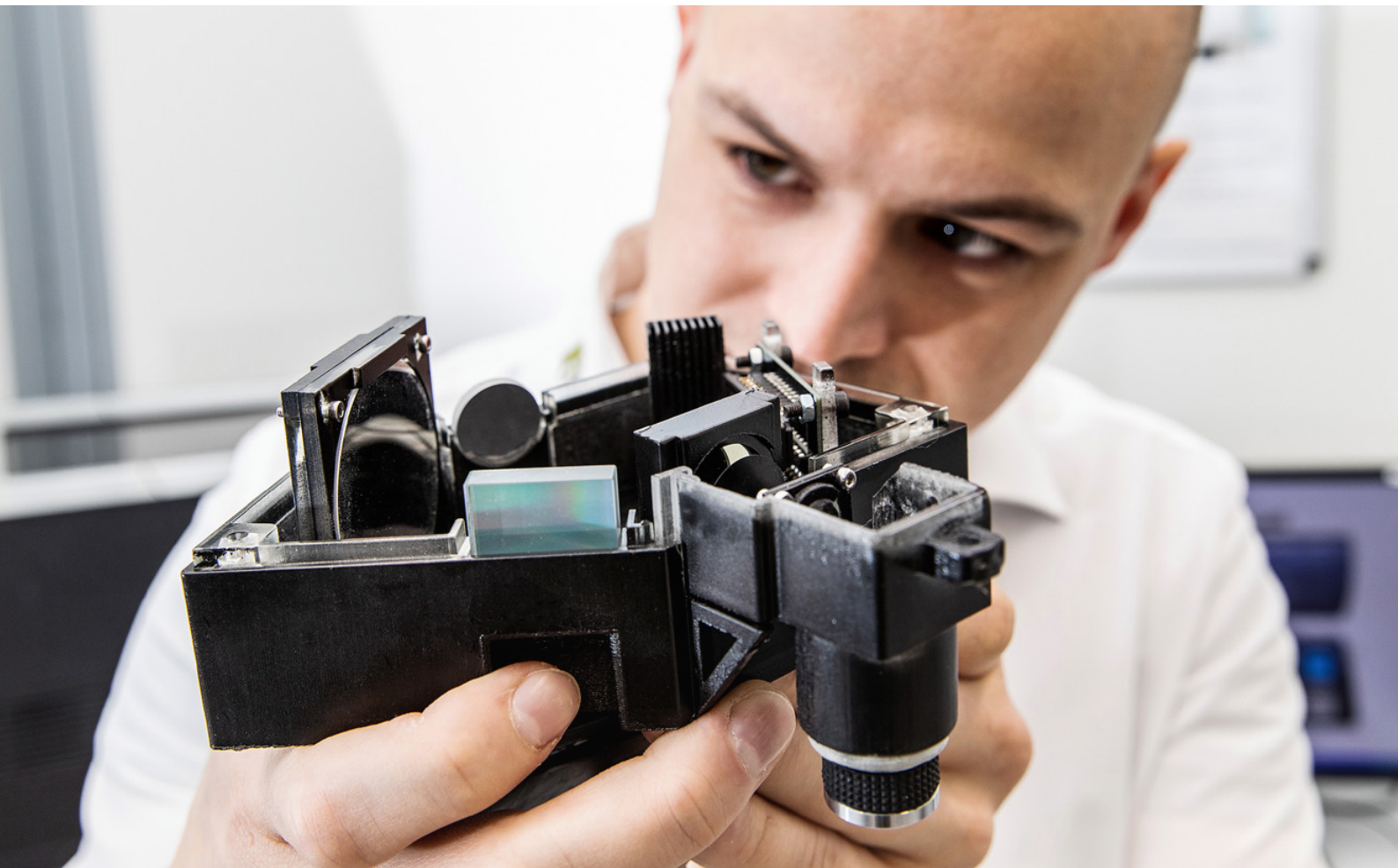
LUH researcher Tobias Grabe holds the prototype of a partially additively manufactured Raman spectrometer in his hands.
