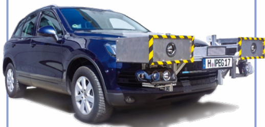
Lighting test vehicle with prototype high-resolution headlamps that use technologies from video projectors.
