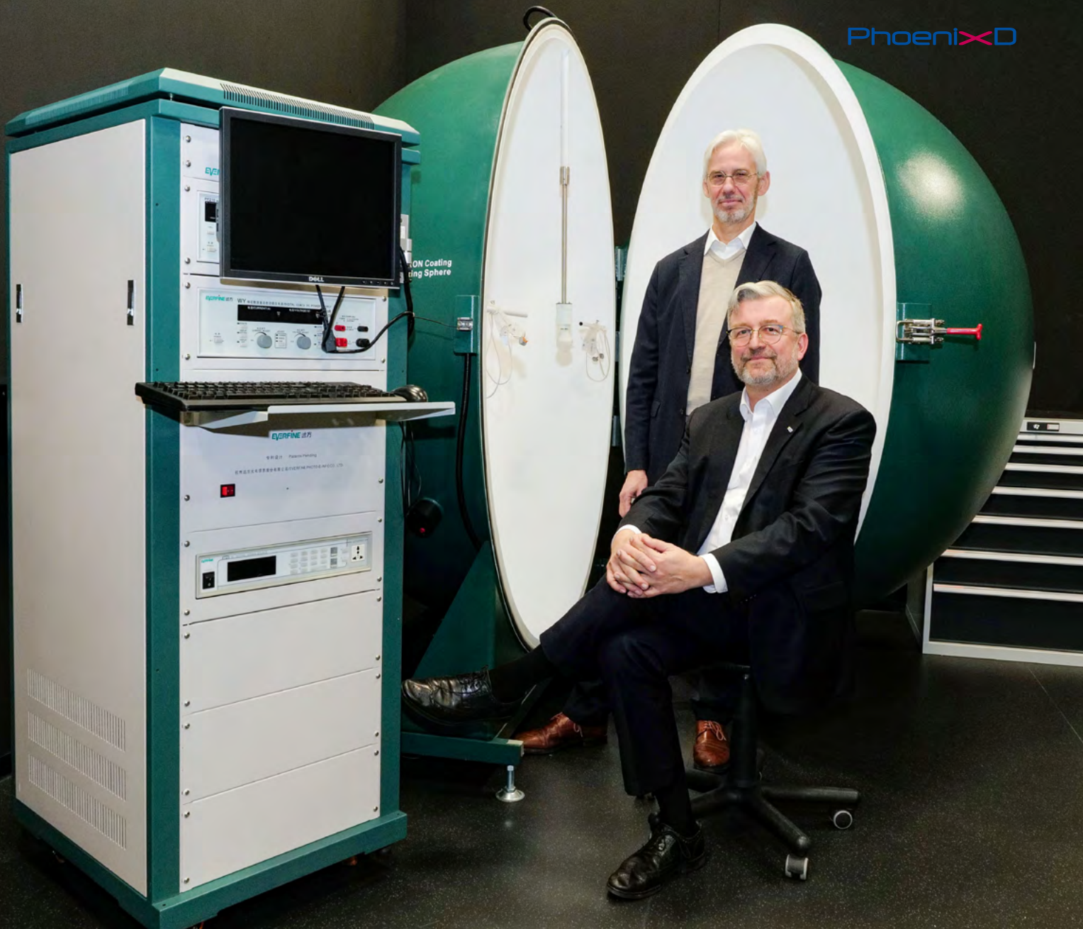
Roland Lachmayer (seated) and Berend Denkena (standing) work at the Mechanical Engineering Campus of Leibniz University Hannover in Garbsen, where scientists use an integrating sphere (Ulbricht sphere) to determine luminous flux and specular distribution.
